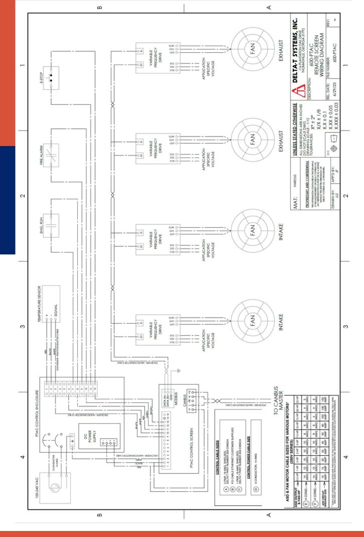
PTAC REMOTE SCREEN WIRING DIAGRAM
