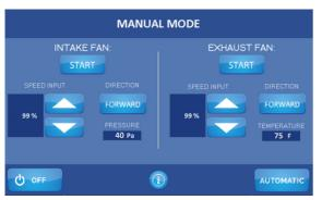
If you would like to operate the vessel in manual mode, click the manual mode button in the bottom right corner, and input the desired settings.
